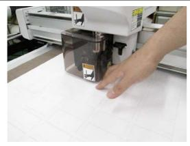
Do not put your hands on the carriage moving path. Avoid suppress the work by hand, please use the absorption sheet always.
